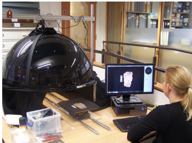
Dr Piquette tests the RTI dome on a lead curse tablet at the CSAD
