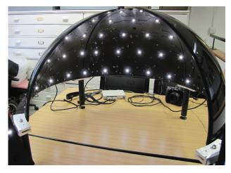
Oxford RTI lighting dome, set up in CSAD, with one quarter removed to reveal the LEDs affixed to its interior surface. The black reflective sphere is used to record the light positions during calibration.
